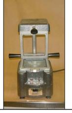
Close the sandwich holder tightly, and raise the material to the top of the bar where the heater is located.
